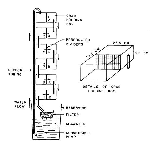
Fig. 1. Recirculating seawater system for the maintenance and feeding of blue crabs.
